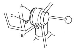
Figure B: Drill Depth Adjustment
